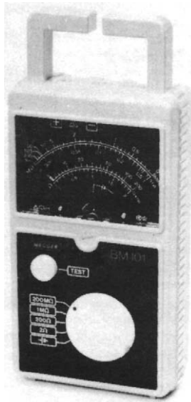
Figure 12.9 Type BM101 insulation and continuity tester (Avo Megger Instruments Ltd)
